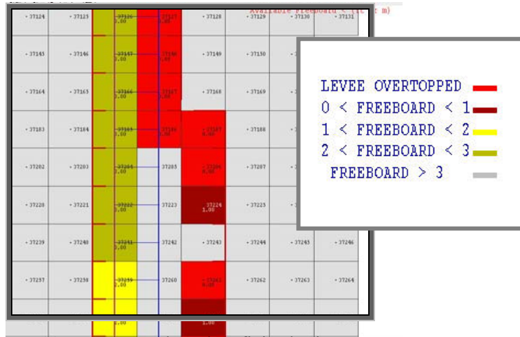
Figure 10. Levee Freeboard Deficit Plot in Mapper
